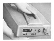
range of exposures. A push-button activates the 3-digit LED display (0-999 mR range). Chirps are emitted in direct proportion to the radiation intensity. Typically, it will chirp once or twice per min in a 1 mR/hr field. The accumulated exposure is cleared by turning the dosimeter off. -Nuclear Associates, Inc., 100 Voice Rd., Carle Place, NY 11514.
