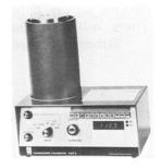
isotopes, the CRC-5 also provides over 90 radioisotope calibrators for manual selection. Available options include a remote calibration detector and a radiation exposure monitor.
