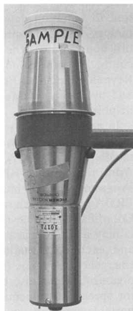
FIG. 1. Collimated 2 x 2-in. NaI detector normally used for thyroid uptakes is inverted and covered with plastic petri dish for doing radioassays on small samples.
