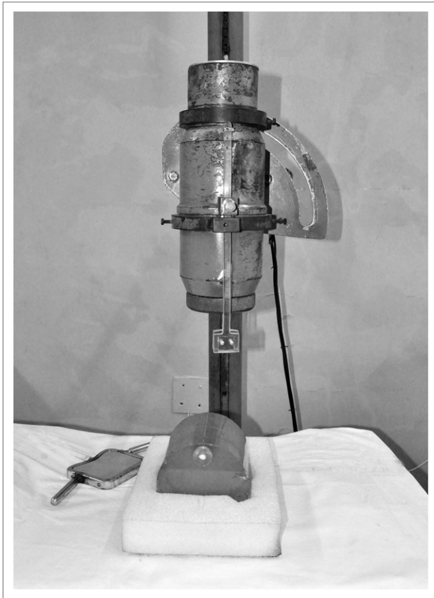
FIGURE 1. Thyroid uptake probe ( ^{131}\text{I} capsule in acrylic glass phantom).
