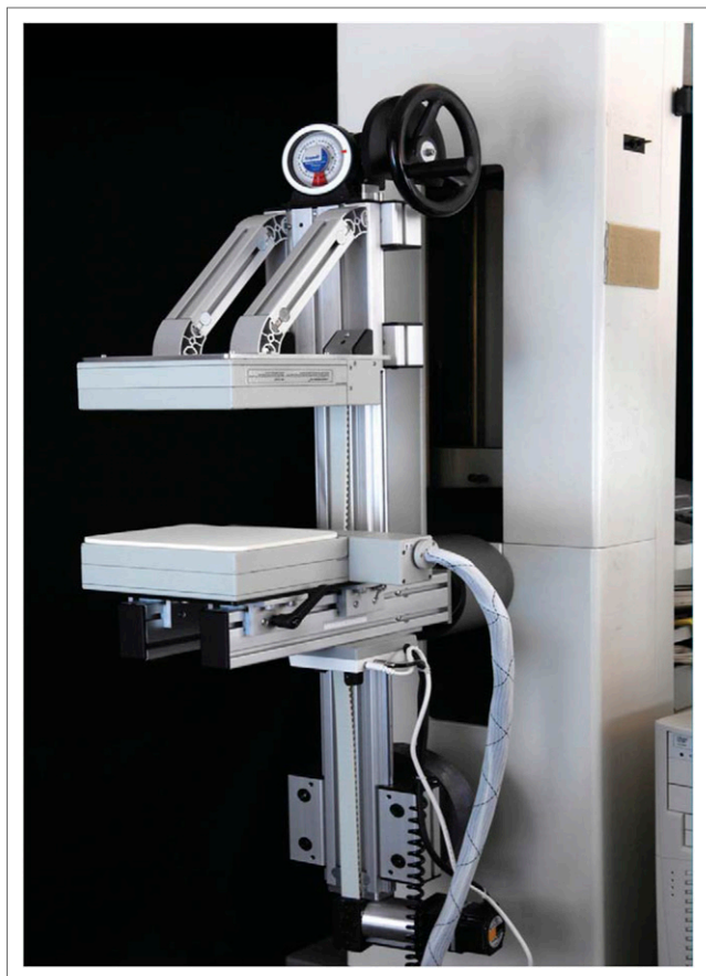
FIGURE 1. Cadmium zinc telluride-based molecular breast imaging camera. (Reprinted with permission of (79).)
