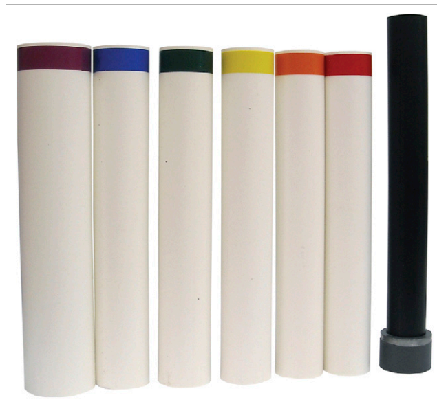
FIGURE 2. Linearity attenuation shields. Source is placed in black tube, which is in turn placed within measuring space of dose calibrator. Other tubes, which have colored bands around upper edge, are then placed into dose calibrator around black tube. Known attenuation factors of each combination of tubes allow operator to simulate activity levels over wide range, thus assessing dose calibrator’s ability to measure accurately at different activity levels. (Photo courtesy of Capintec, Inc.)
