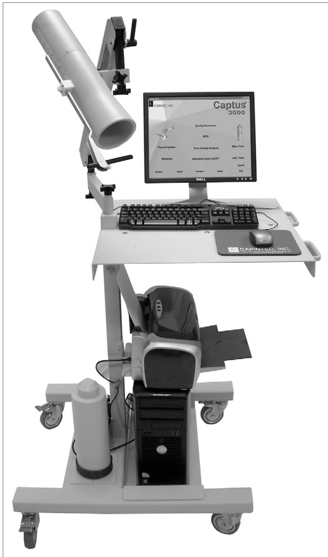
FIGURE 4. Thyroid probe/well counter. This instrument contains 2 detectors, organ probe at upper left and well counter at lower left, sitting atop base/wheel assembly. Both detectors use sodium iodide, a scintillation crystal, as the detection material, and both produce an energy spectrum as their output. Scintillation detectors have an inherent advantage over gas-filled detectors, in that the detecting material is much denser and therefore more likely to interact with \gamma rays and other high-energy photons. (Photo courtesy of Capintec, Inc.)
