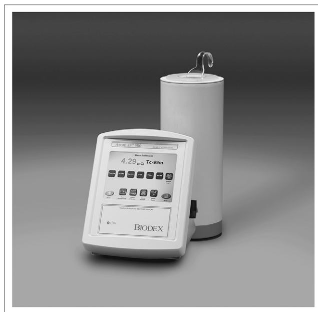
FIGURE 1. Dose calibrator. Electronics module almost always sits separately from cylindric ionization chamber, as shown in this figure. Ionization chamber is surrounded by lead shield, which blocks external radiation from entering and also causes photons from source being measured to be backscattered into gas space. Dipper handle can be seen coming out of measurement space. (Photo courtesy of Biomedex Medical Systems, Inc.)
