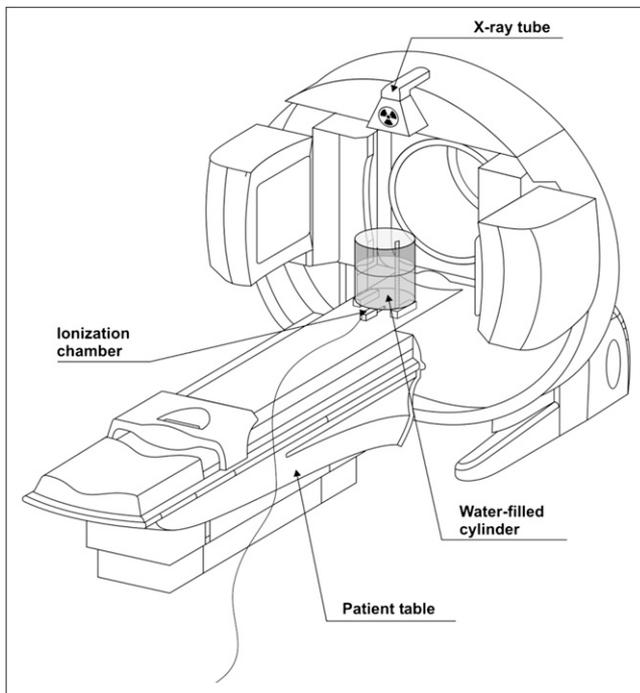
**FIGURE 1.** Schematic illustration of exit dose measurement geometry.
