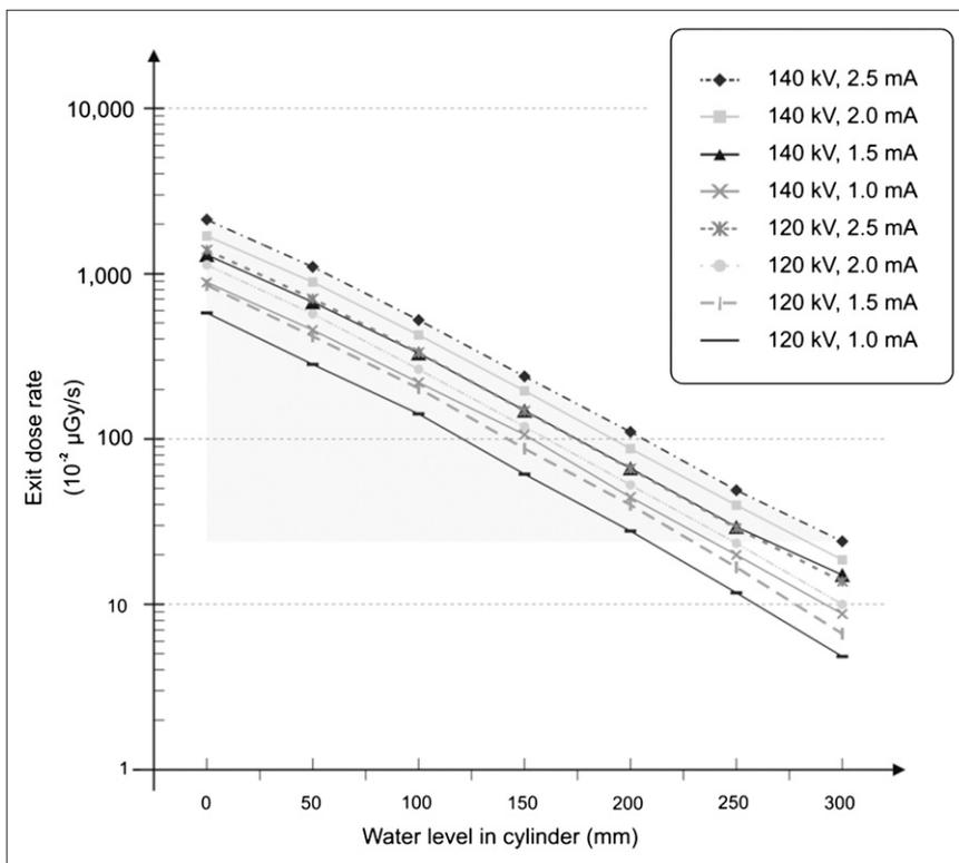
**FIGURE 2.** Semilogarithmic graph of exit dose rates for various voltages and currents vs. increasing depth of water in phantom simulating attenuation in patient.
