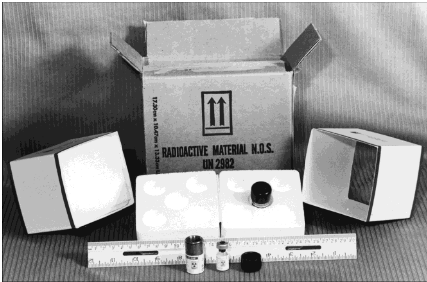
FIGURE 1. Packing materials for a shipment of 2 ^{133}\text{Xe} vials. Each vial is packed in separate polystyrene packing materials that consist of 2 halves with 5 holes that can house up to 5 shielded ^{133}\text{Xe} vials. A single vial is placed in the center hole. Each set of packing materials is placed in a cardboard sleeve to hold the 2 halves together.
