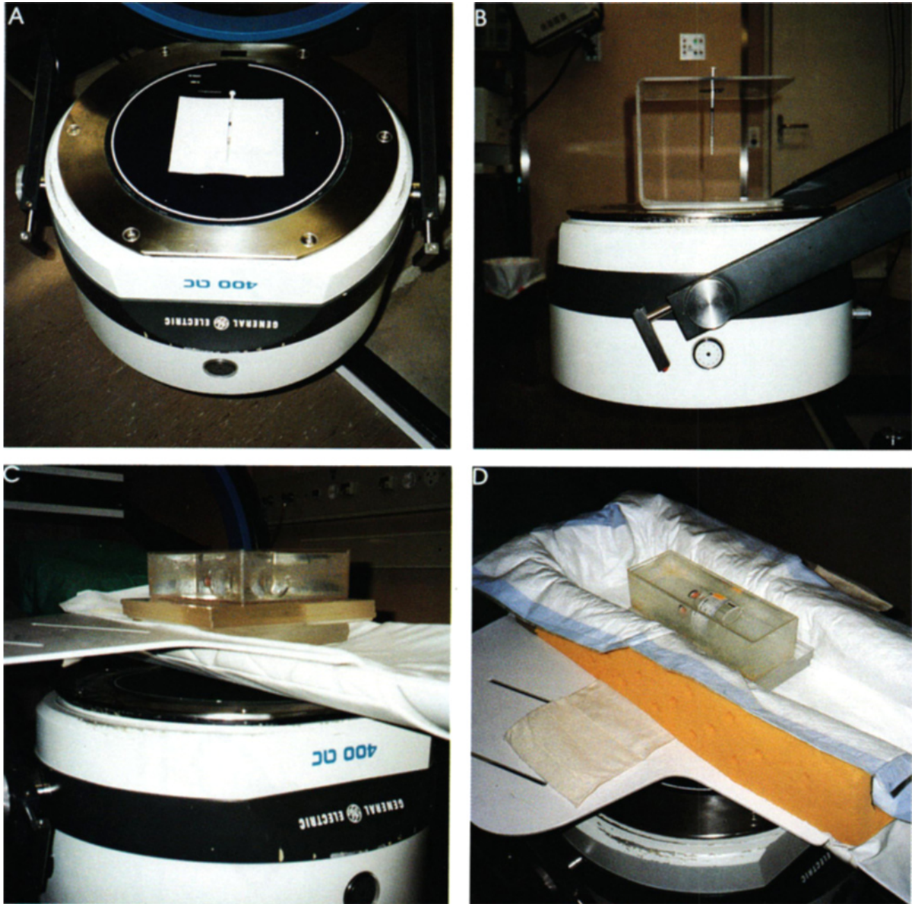
FIG. 4. Measurements of injected activity: (A) the contact method, (B) the 24-cm distance method, (C) the phantom method, and (D) the phantom method in infants.
