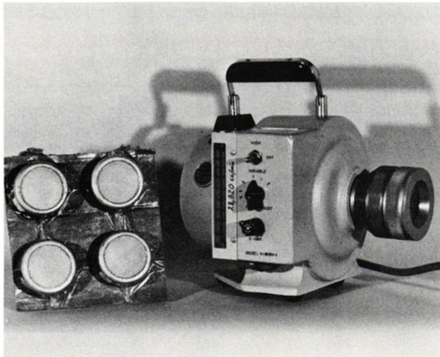
**FIG. 1.** Air pollution sampler and charcoal cartridges used in monitoring I-131 air exposure levels during radioiodine preadministration and administration phases.
