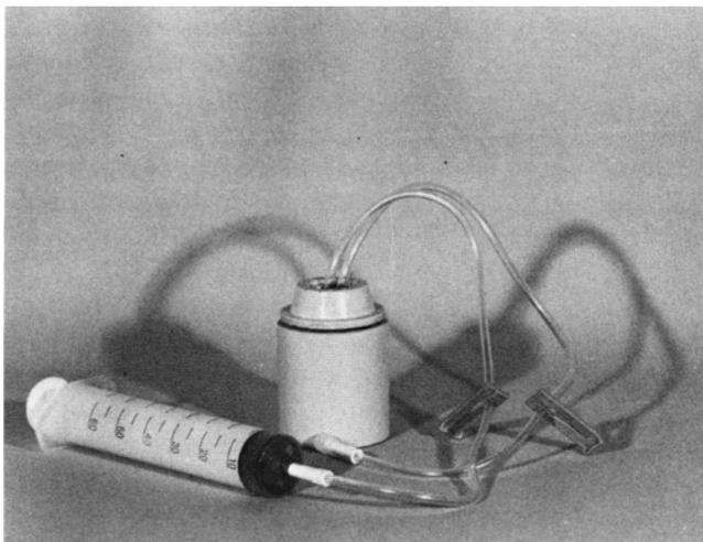
**FIG. 3.** Experimental radioiodine administration device (30-cc clear glass vial with venotubing and 60-cc luer-lock syringe) as it would appear secured inside generator solution shield.
