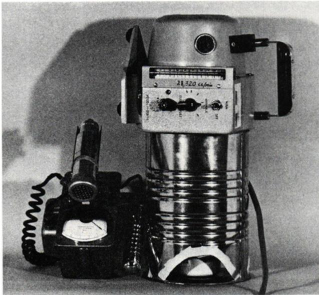
**FIG. 4.** G-M survey meter and air pollution sampler as they were positioned next to and within cylindrical metal can during the radioiodine preadministration and administration phases.
