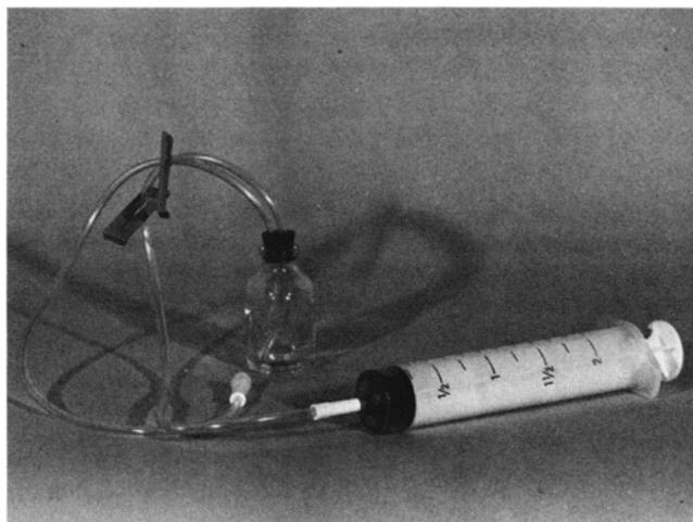
**FIG. 2.** Experimental radioiodine device (30-cc clear glass vial with venotubing and 60-cc luer-lock syringe) as it would appear without generator elution vial shield.
