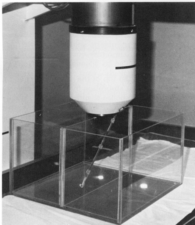
FIG. 1. 45-deg line source used for collimator comparisons.
