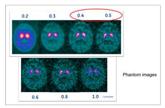
**FIGURE 7.** DaTscan study with different filter settings. Cutoff of 0.4–0.5 is usually good, depending of type of SPECT camera. Once interpreting physician chooses filter setting, it should be applied consistently for each study. (Courtesy of Liz Clarke.)
